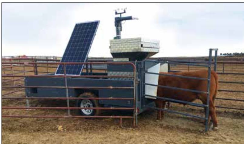
These units at Olsen Ranches, Harrisburg, Neb., collect individual methane emissions for the collaborative research project between the AHA and Colorado State University.
