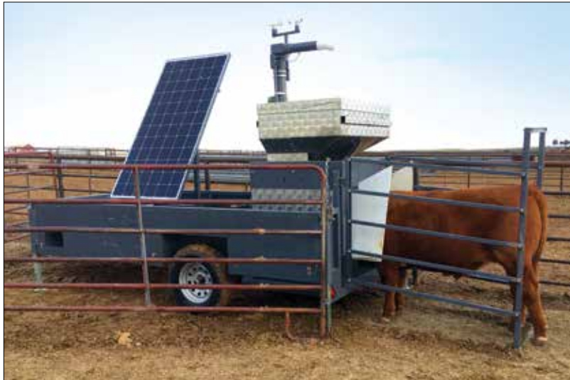
The American Hereford Association is working with AgNext and Colorado State University to identify genetic relationships associated with cattle greenhouse gas emissions. These units at Olsen Ranches, Harrisburg, Neb., collect individual animal methane emissions.
