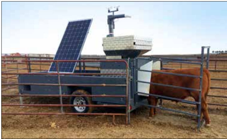
These units at Olsen Ranches, Harrisburg, Neb., collect individual methane emissions for the collaborative research project between the AHA and Colorado State University.
