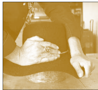
Blocking is the process where Kaycee begins working the owner's unique head shape into the hat.
