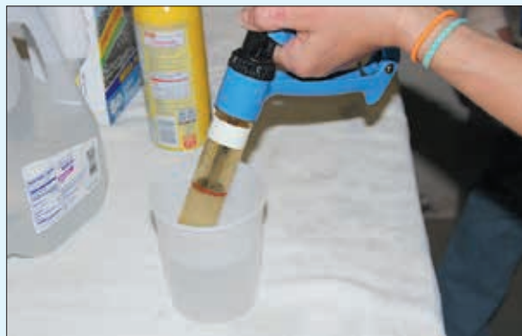
4. Draw up boiling hot distilled water into syringe and squirt it. Repeat three times.
